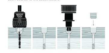
**Screw and Plug:** The other accepted method for a hidden fastener look is the Starborn ProPlug system, as it still achieves face screwing for maximum hold-down and the use of stainless steel screws.
