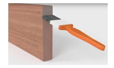
End Sealer: Nova Decking is always end-sealed during manufacturing to help prevent splitting and checking on the ends of boards. We require that the boards are end-sealed as soon as possible after making any cuts to the boards. A clear, water-resistant wax should be used. One such product is Anchorseal 2 from UC Coatings, although several other products are available. If the material is not end sealed the manufacturer will not honor any claims under the warranty.
